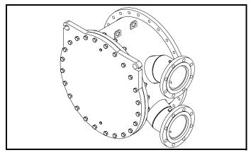
**Flanged connection option** provides an ANSI (American National Standards Institute) flange on the end of the chiller water piping for connection to a customer supplied mating flange in the field piping. This option is available for both the evaporator and condenser.
